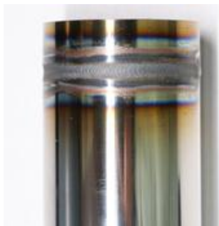
溶接施工例 (φ50.8mm/t3.0mm)
